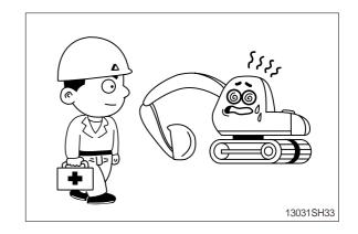
Park on a flat place and stop the engine for inspecting and repairing. Properly TAG machine is not operational. (Remove start key)
