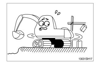
When using the machine as breaker or working in a place where stones may fall down, cab roof guard and head guard should be provided for proper protection.
